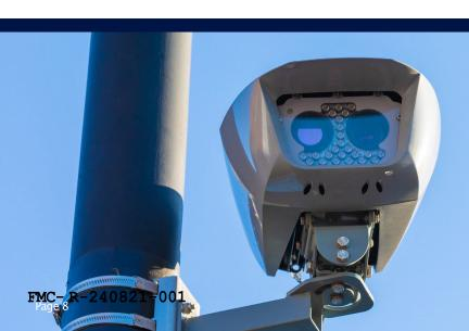
This e-screening technology is positioned ahead of a weigh/inspection station to **notify CMV drivers** of their eligibility to bypass the enforcement location.
